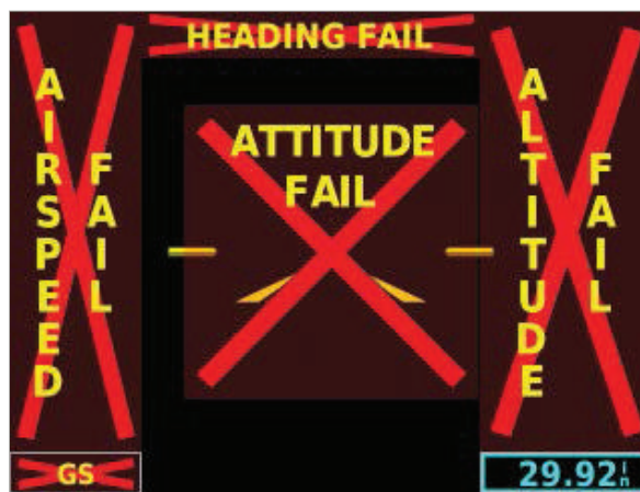
Figure 1-2 G5 PFD Page Failure Annunciations
