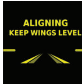
Figure 1-5 Attitude Aligned Keep Wings Level Indication
