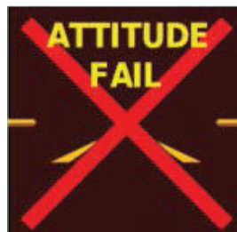
Figure 1-6 Attitude Failure Indication
