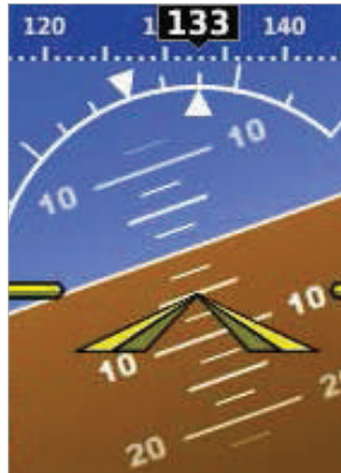
Figure 2-7 Ground Pointer Configuration
