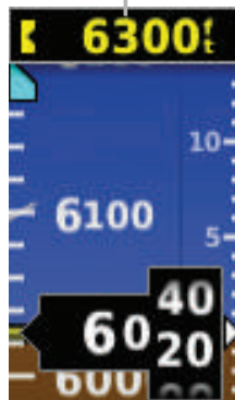
Figure 2-10 Altitude Alerting Visual Annunciation
